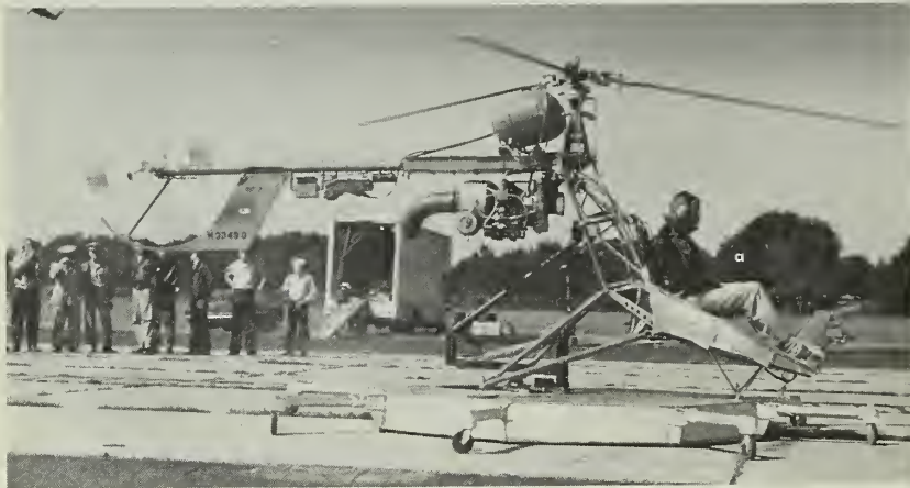
JET TURBINE helicopter, called a Whirly-Mite , is demonstrated for helicopter pilots at Ellyson Field, Pensacola. Platform prevents flights over three feet.
